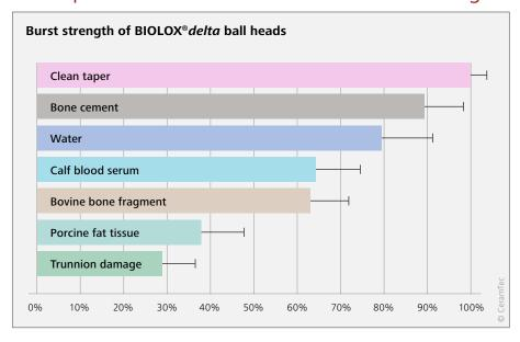
The burst strength of BIOLOX® delta ball heads is reduced when these materials contaminate the stem taper.
