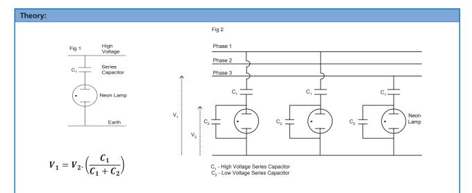
In it's simplist form the Live-Line Indication consists of a high voltage ac rated capacitor which is connected in series with the neon indicator between the phase and earth lines. (Fig1).
