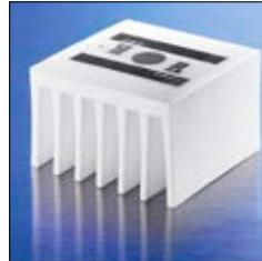
CeramCool® geometry for 4W cooling. With Rubalit® the total thermal resistance  $R_{tt}$  of the assembly is at least 13% better than aluminum. Using Alunit® it is more than 31% better.
